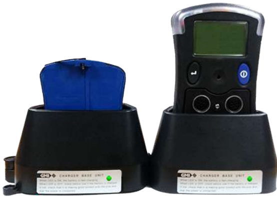
Long duration battery pack & instrument with fast charge battery pack, charging in Fast Charger master / slave units.
