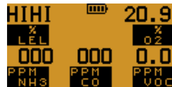
Display in alarm conditions
