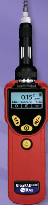
The UltraRAE 3000 is the most advanced Compound-Specific Monitor on the market. Its Photoionization Detector's (PID) extended range of 0.05 to 10,000 ppm in VOC mode and 50 ppb to 200 ppm in benzene-specific mode makes it an ideal instrument for applications, from entry pre-screening during refinery and plant maintenance to hazardous material response, marine spill response and refinery down-stream monitoring.
